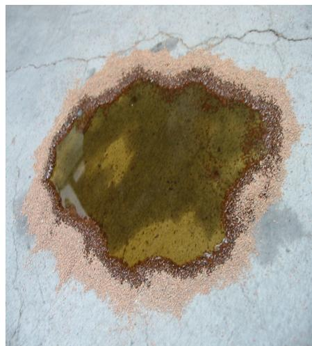
**MIXI grain acts as a barrier to the propagation of spilled oil**
